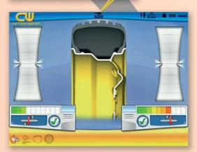
While two vehicles may be similar in terms of size and weight of wheels and therefore have similar moments of inertia, they clearly need different and specific wheel balancing solutions, as the imbalance effect is proportional to the square of the speed.
