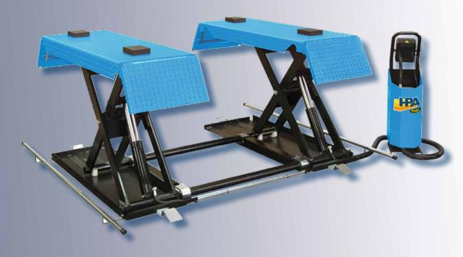
Reversible low-profile electrohydraulic scissors lift for **cars, SUVs and vans**; ideal for tyre specialists, car workshops, and body repairers. Runway levelling guaranteed by 2 sturdy anti-torsion connection bars. Low voltage control unit with **"dead-man" control system**. Available in on-floor and flush installation versions.
